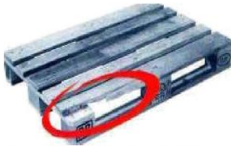
A floor or deck-board edge is splintered off so much, more than one nail is visible.
